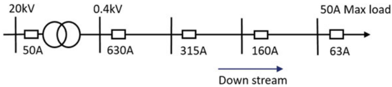
Fig. 26.6 Radial feeder protection using fuses
